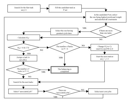
Figure 1. Single model line balancing procedure
