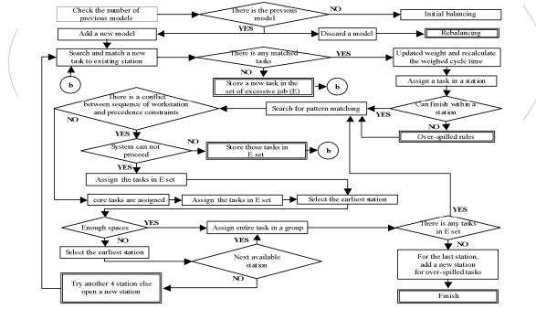
Figure 2. Mixed model line balancing procedure
