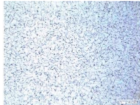
Micrograph of base metal of TRU-02-1
