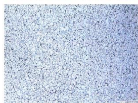
Micrograph of heat-affected zone TRU-02-1
